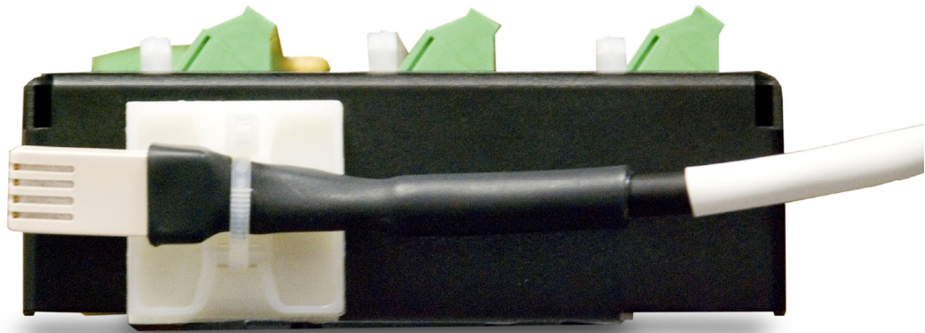
FIGURE 1. CS210 Installed on a CR1000
